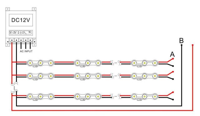
A. Max. number of modules in one chain when the power supplied from single end -50pcsB. Max. number of modules in one chain when the power supplied from both ends -100pcs
