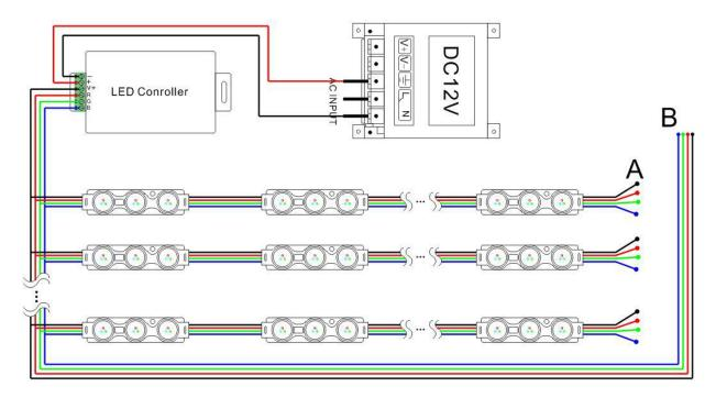
A. Max. number of modules in one chain when the power supplied from single end -20pcs B. Max. number of modules in one chain when the power supplied from both ends -40pcs
